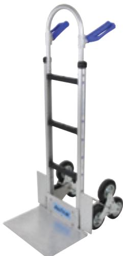
The heavy duty **stair climber truck** has two sets of three triangular set wheels which rotate to climb steps. It has a solid extended 405x305mm foot for bulky items and weighs only 18kg. Capacity is 180kg when climbing or 300kg on ground level.
